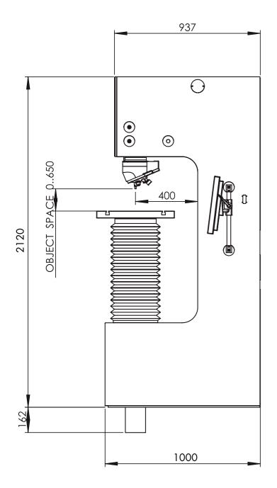
All dimensions in these drawings are in mm, approximate. Working heights and or workpiece accommodation varies depending on the stages and stage accessories used.
