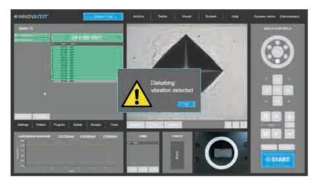
For certain countries/area's in the world where light earthquakes are so common that they are hardly noticed, the vibration monitoring system will give a warning message and stop the hardness testing process to avoid incorrect readings.
