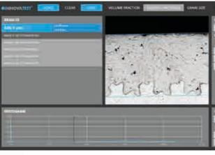
The FALCON 600G2 is basically an upright, brightfield and darkfield microscope. Contrast methods of reflected light brightfield result are best suited to analyze the microstructures of etched surfaces. Recognizing grain boundaries, you can draw conclusions on grain sizes, phases and structural constituents. Impurities and structural constituents, such as graphite in cast iron, prior to etching are getting visible.
