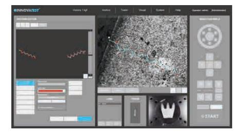
The distances of test points are automatically set to a minimum distance, following the standard, to assure correct testing is conducted. Time saving test mode "complete all indentations – then evaluate" and "auto-stop" to complete test series as soon as the lower hardness limit has been reached. Report Generator is enhanced with reporting features for this application.
