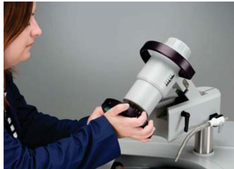
Kick-stand holds head in place for easy installation of specimen holder.
