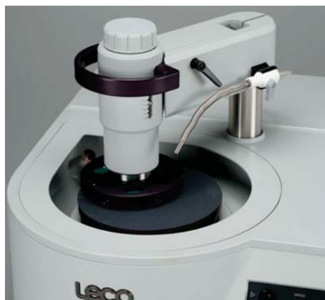
A simple turn of the head's top knob adjusts the force applied to the specimens.
