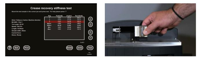
Rounded corner crease resistance: Rounded corner creases can be tested on the CFA (requires additional jaw).
