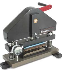
Prepares individual crease and stiffness samples. Suitable for low-medium volume testing.
