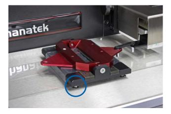
Lift pins retract into the instrument and the sled is placed in the same position each time  $% \left( {{{\rm{D}}_{\rm{s}}}} \right)$
