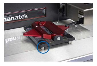
Sled is positioned on lift pins
