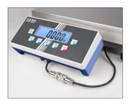
Verification plug, for verified balances this enables you to separate the display device and platform without affecting the verification, e.g. for installing the scale in a packing and dispatch table, pit frame etc. at a later date.
