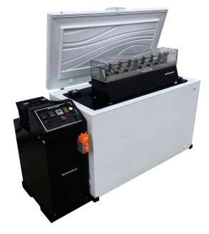
button pendant is located outside the freezer to operate the lift.
