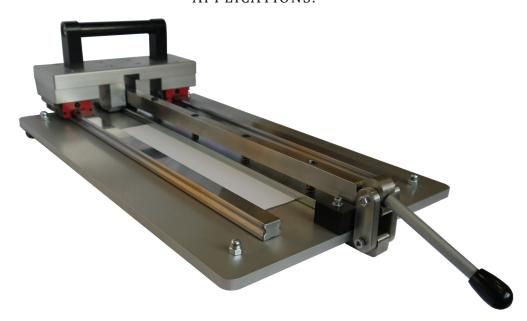
The cutter has two blades mounted to a separate holder and therefore can be replaced easily when blunt. The blade holder is mounted onto a draw down carriage which is guided and running on two rails, this ensures parallel running and precise cutting.
