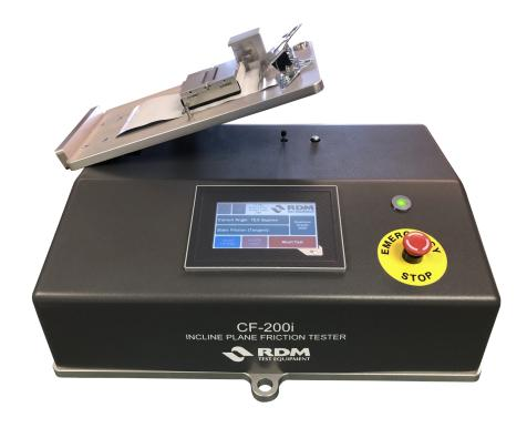
Slide angle friction is a measurement of a sheet like substrate such as paper, plastic film, thin board, corrugated board etc. which determines the angle of inclination at which one substrate affixed to a sled will begin to slide/slip against another substrate of a similar material affixed to a bed.
