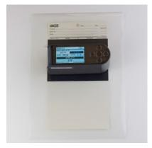
Measurements are made over a white substrate and then over a black substrate. Opacity is automatically calculated and displayed.
