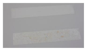
Clear tape is pressed on the measurement surface, torn away and stuck onto white paper - For reference a clean piece of tape is also stuck on the same white paper.
