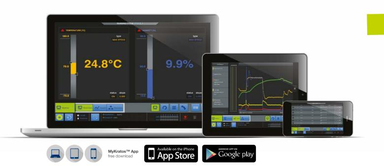
It is possible to have **multi-users** and **multi-level connections**, even coming from different devices. Once the chamber goes into execution mode, the user that started the test becomes its sole manager, allowing others to consult it in readonly mode and to set the subsequent cycles. All data are saved inside the chamber built-in datalogging, so they are always available to the users regardless of the device used.
