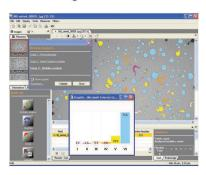
IMAGIN NODULA 200 module is designed for the analysis of graphite in cast irons especially in Ductile and Gray Iron Foundries and Quality Control Labs. Nodularity assessment is made by percent count and nodules proportion. It is also possible to measure "Area percent ferrite, Area percent graphite and Area percent Pearlite". Archiving of all images with calibration and generating Reports creates an additional advantage to increase productivity and repeatability.
