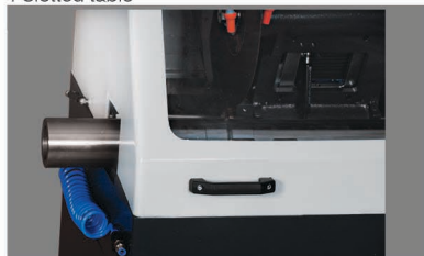
Side access port for extra-long workpieces
